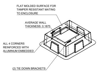
FIBERGLASS BOX PAD REINFORCED WITH ALUMIUM EMBEDEED 43" WIDTH X 37"DEEP X 15" HIGH WITH 24" X 22" OPENING. INCLUDES HOLD DOWN CLAMPS.
